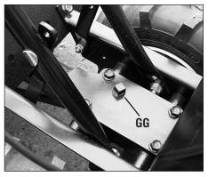
Fig. 2-11: Remove gear oil fill plug.
